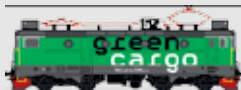
Name: Rd Number: 44 Comment: All equipped with radio control, 130km/h Rated power: 3.6 MW
