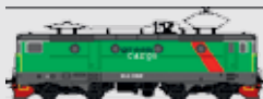
Name: Rc4 Number: 121 Comment: 62 equipped with radio control, 130km/h Rated power: 3.6 MW
