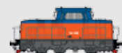
Name: V4 Number: 3 Comment: All equipped with radio control (40/70 km/h) Rated power: 0.460 MW
