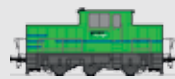
Name: V10 Number: 2 Comment: All equipped with radio control Rated power: 0.485 MW
