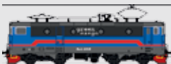
Name: Rc1 Number: 16 Comment: All equipped with radio control, 130km/h Rated power: 3.6 MW
