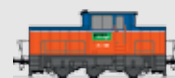
Name: V5 Number: 40 Comment: All equipped with radio control Rated power: 0.380 MW
