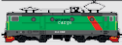
Name: Rc3 Number: 3 Comment: 2 equipped with radio control, 160 km/h Rated power: 3.6 MW
